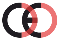
False CE Mark (too close)
